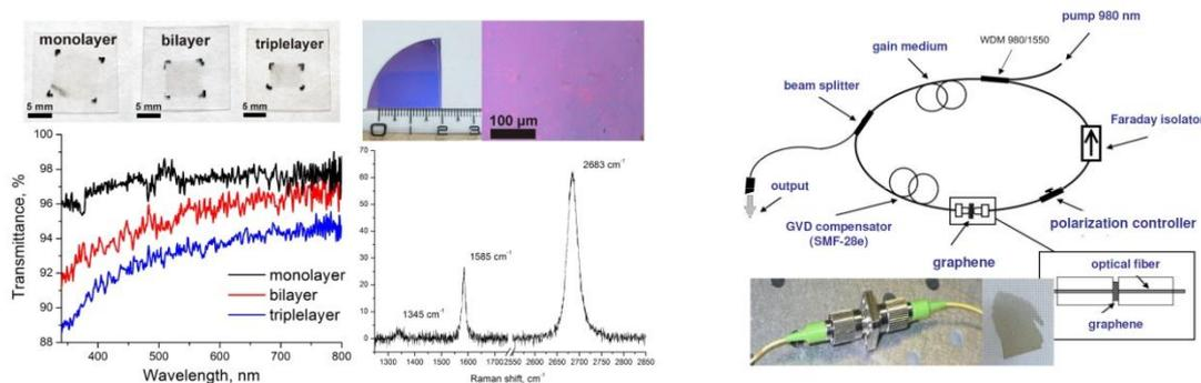
Fig. 1. Photographs of graphene on glass and Si/SiO<sub>2</sub> substrate and its optical absorption spectra and Raman spectrum (left). Scheme of mode-locked laser with graphene saturable absorber (right).
